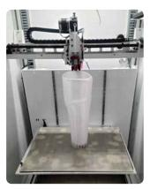
3D printing has emerged as a game-changer in the prosthetics and orthotics field. Leimkuehler, Inc. has been 3D printing prosthetic diagnostic sockets, also known as test sockets. These test sockets are a temporary prototype of the final prosthetic socket. This allows us to ensure a comfortable and secure fit for our patients. This technology is revolutionary as it leads to a better fit, reducing office visits for our patients, and leads to a faster delivery of their final prosthesis.
